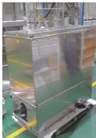
Vacuum vessel and thermal shield of QWR Cryomodule for SRILAC at RIKEN RIBF
